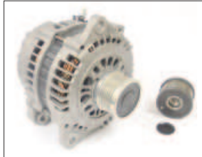
Figure 3 - A 13939 alternator and its clutch pulley
